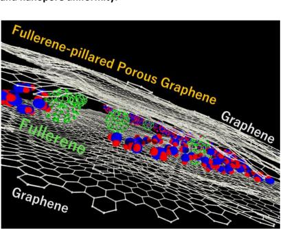
Image title: Fullerene-pillared porous graphene fabricated by a bottom-up process.
